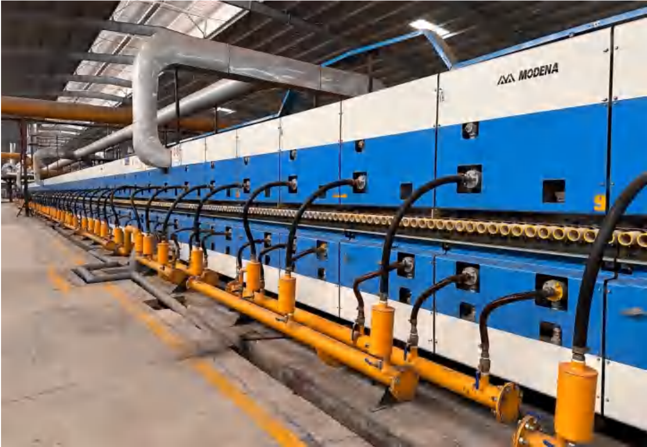
Customer: HERA INDUSTRIAL JOINT STOCK COMPANY Project: Glazed Roof Tiles Equipment supplied: Firing Kiln mod.MFS , 5-Layer Dryer mod.MRD-H5 Product and output: 14x310x340MM, 340x360MM; 6,000sqm/D 工程内容: 屋顶西瓦 主要使用设备: MOD. MFS烧成窑炉, MOD. MRD-H5 五层干燥窑 产品类型及产量: 14 X 310 X 410MM, 340 X 360MM; 日产6,000平方米
